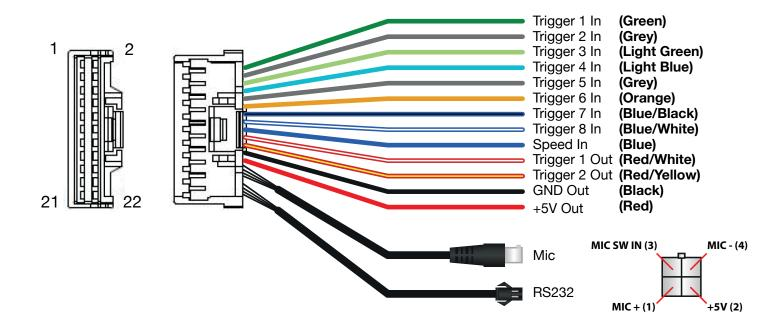
**Trigger IN:** 1-8 can be a high or low trigger value which is configured in the menu of the DVR
